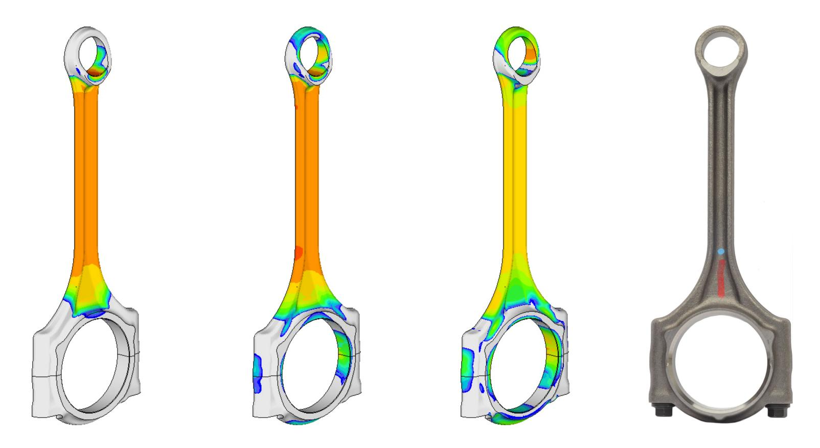
The weight of the new connection rod was reduced by 31%. The old connecting rod total mass was 1488 grams (two rods) and the new • MAHLE design is 1020 grams (two rods). Additional weight reduction will be achieved by adjusting the crankshaft counterweights for mass balancing (customer responsibility).
